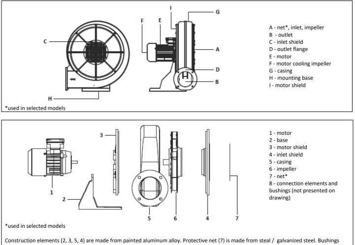
and connection elements are made from steel, galvanized steel, stainless steel. For sealing - sealing paste and or sealing tapes has been
