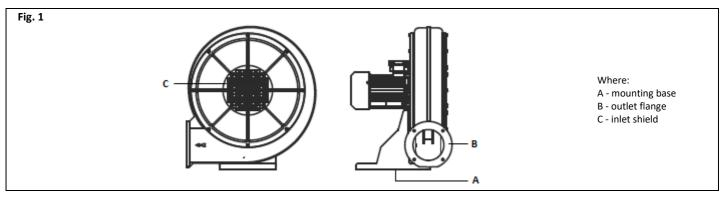
•Supporting construction has to be solid enough in order to carry the weight of the fan and generated vibration (including fan damage). The fan cannot be exposed to vibration.
