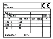
Connection in Y 3x400V 110Hz system only, maintaining the settings for the frequency converter.
