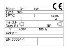
Connection only in Y 3x400V 100Hz system, keeping the settings for the frequency converter.
