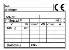
Connection in  $\Delta$  3x400V 100Hz system only, maintaining the settings for the frequency converter.
