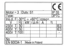
Triangle connection at 3x400V 100Hz while maintaining the settings for the drive.
