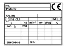
Connection in  $\Delta$  3x400V 200Hz system only, maintaining the settings for the frequency converter.
